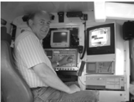
The ABA's Ian Anderson measuring the field strength of the received television signal, and assessing the picture quality of the television program on the monitor.
