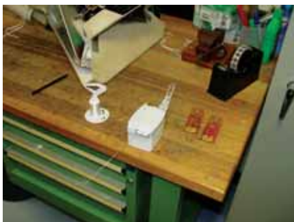
The cause of the interference to Brisbane's CLEM7 tunnel: a small transmitter located inside a meteorological balloon.
