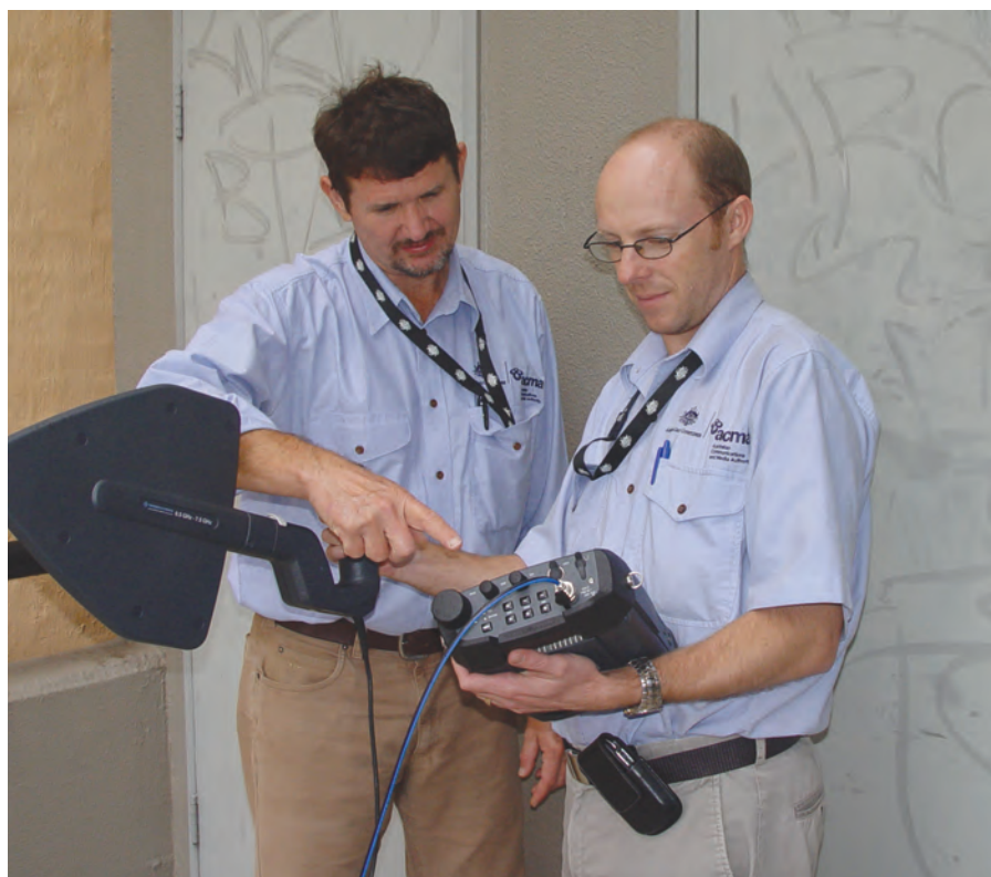
ACMA Field Operations officers Cameron Bell and Michael Cooper using the new Rohde and Schwarz PR100 receiver.
