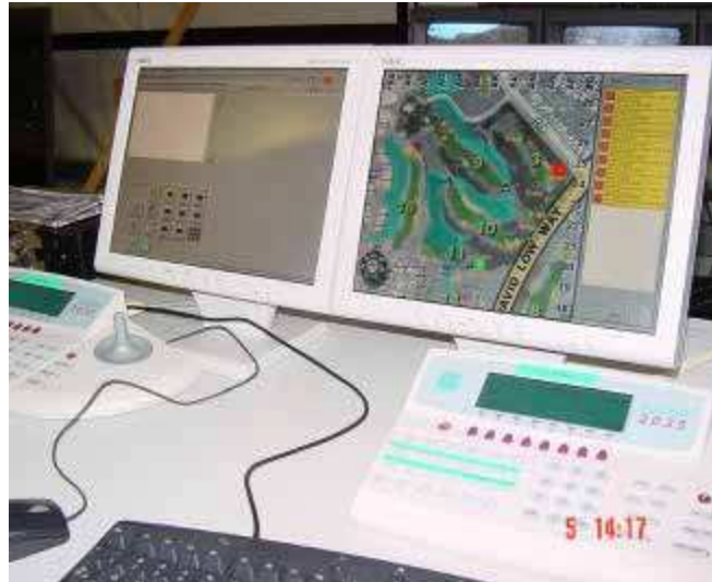
In the field, a series of sensors, acoustic cable and long and short range sensors formed a continuous perimeter around the secure sector. Generally two operators from the ADF monitored the screens and when any of the sensors were activated they flashed on a grid map on a large digital plasma screen.
