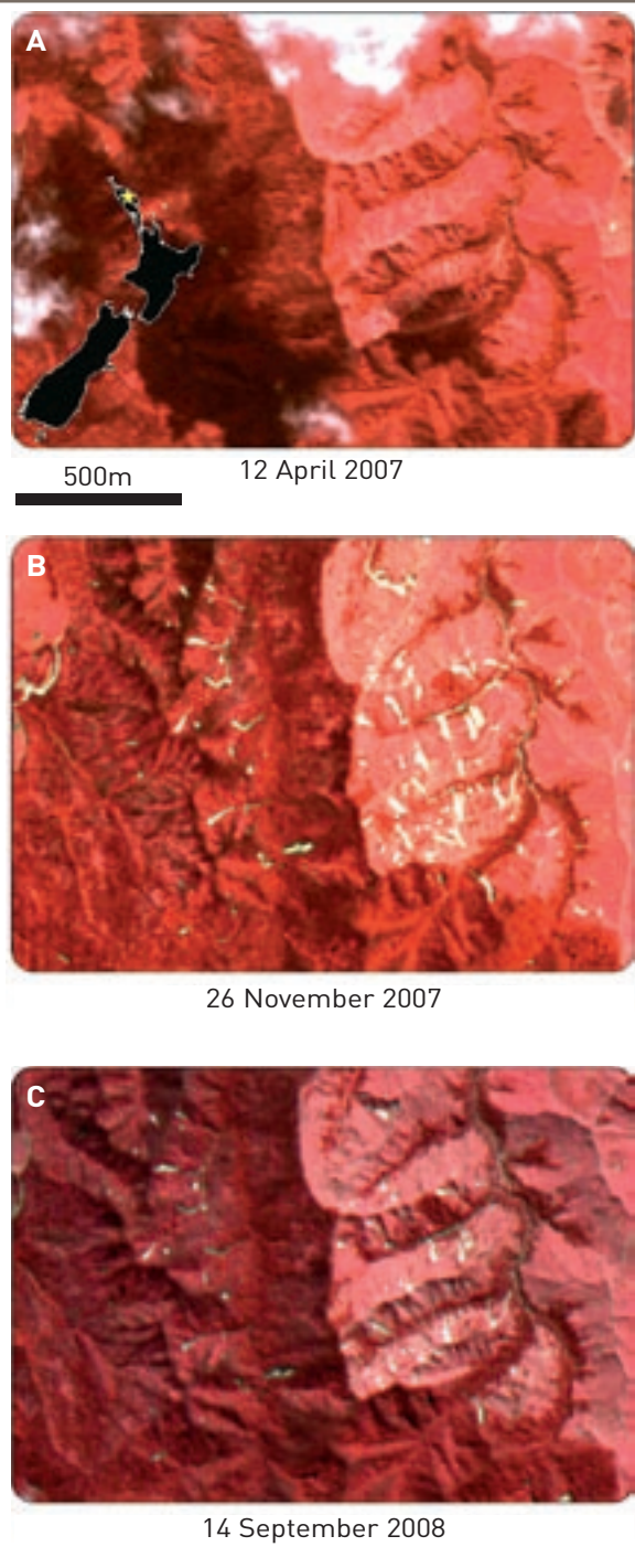
FIGURE 6. Recovery of vegetation after a widespread landsliding event in northern New Zealand, July 2007. (a) SPOT-5 CIR obtained before the event; (b) SPOT-5 CIR obtained shortly after the event; (c) ALOS AVNIR-2 CIR imagery obtained one year later.
