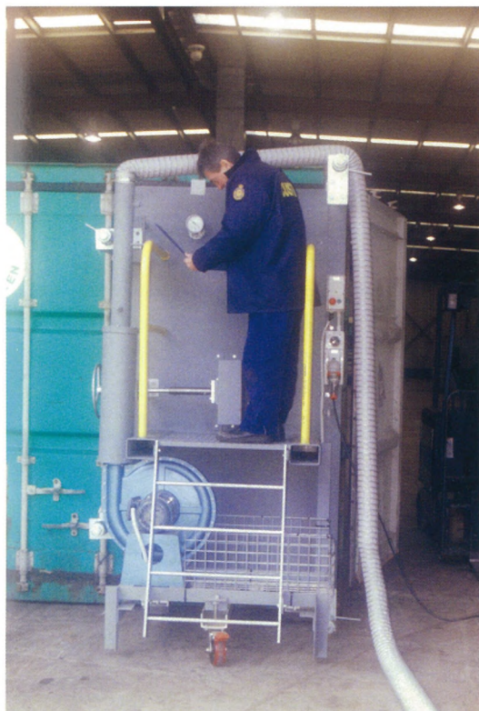
top right: Safety equipment used as a precaution against the absorption of toxic vapours encountered in fumigated cargo containers.
